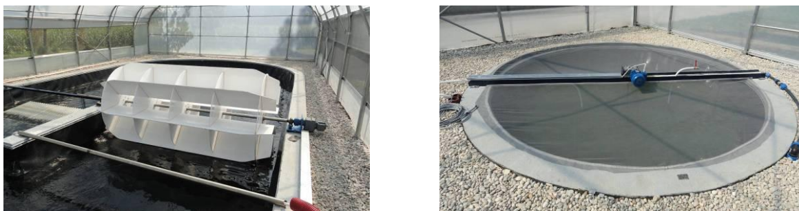
Figure 7 Paddlewheel and vertical mixer in inoculation pond
