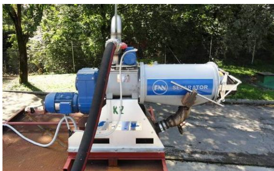
Figure 22 Press Screw Separator and roll-off digestate equalization container
