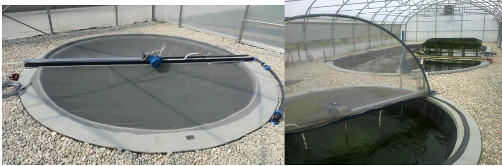
Figure 2 Vertical mixer in inoculation pond, inoculation culture
