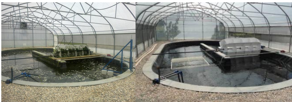
Figure 1 Main pond with paddlewheel mixer on the right and diffuser on the left (M36 and M31)
