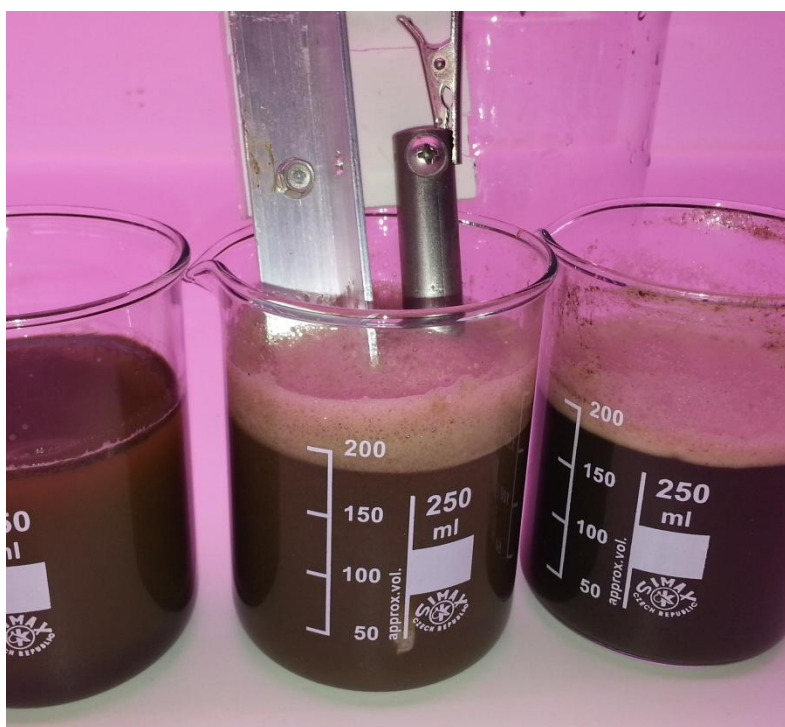
Figure 13 Al-Ti electrocoagulation after approx 20 s
