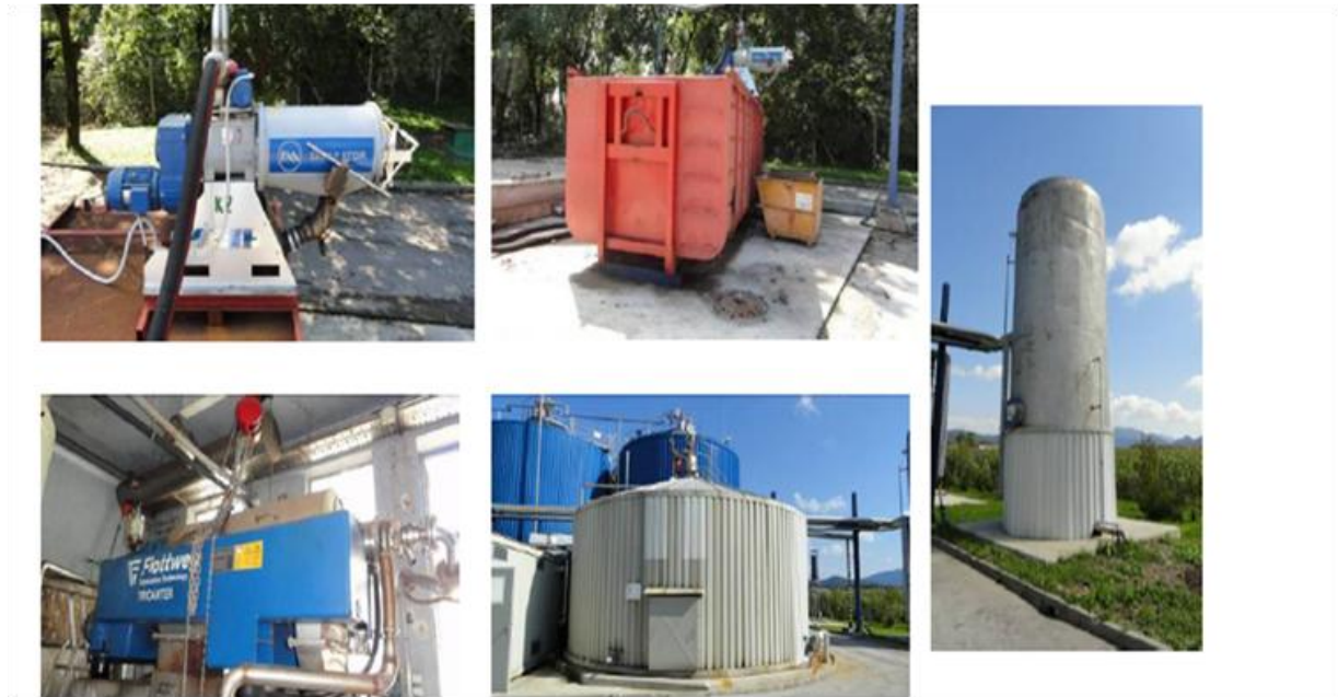
Figure 3 Digestate treatment- from top left to bottom left: fan separator, digestate container, tricanter centrifuge, anaerobic filter (AF), cooling tank (CT)
