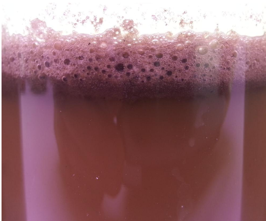
Figure 12 Quick performance of Al-Ti electroflocculation: significant amount of particles flotates after just 30 s treatment
